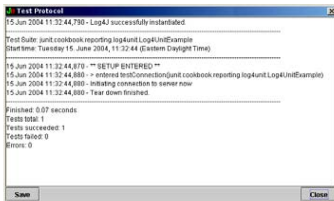
Figure 7.2 The Log4Unit Test Protocol dialog box, showing log statements and test summary information
